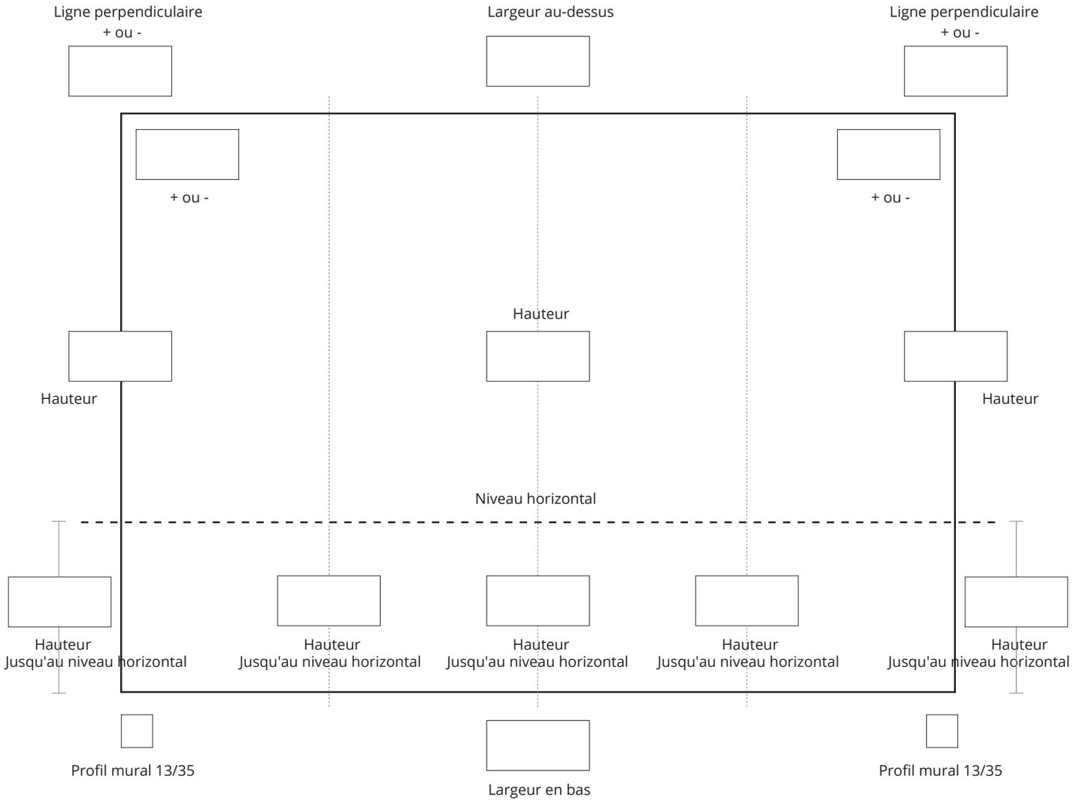
Diagram illustrating the measurement points for a door frame installation. The drawing shows a central door frame with various measurement points and labels:
